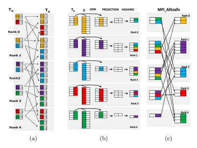
Fig. 6: (a) Intra-bucket communication; each subbucket of  $T_{\Delta}$  sends its data to all subbuckets of G. (b) Local, per-subbucket joins (including projection and re-hashing). (c) All to all communication.
